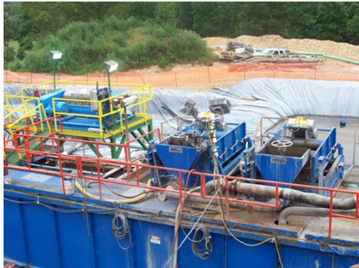
Two NOV linear shakers on right w/centrifuge to the left
